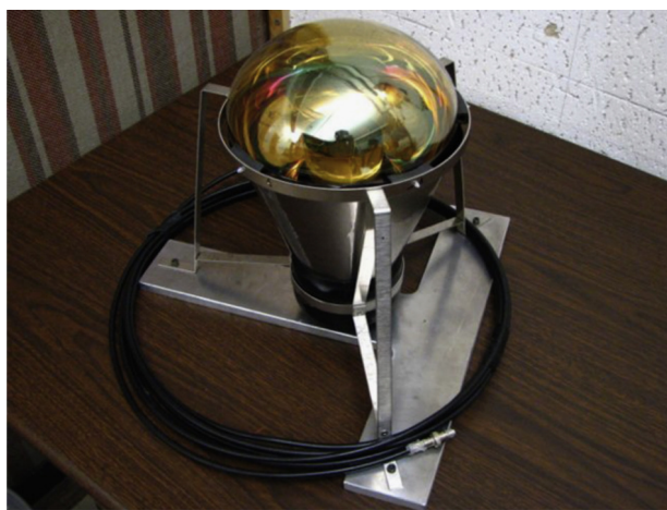
(a) PMT assembly from Daya Bay.
